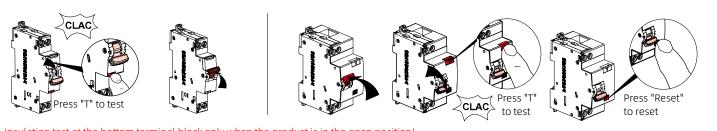
Insulation test at the bottom terminal block only when the product is in the open position!
