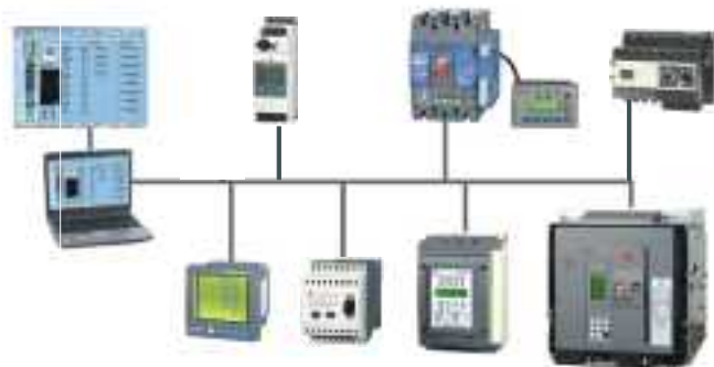
● Ri year-PowerNet配电监控系统
